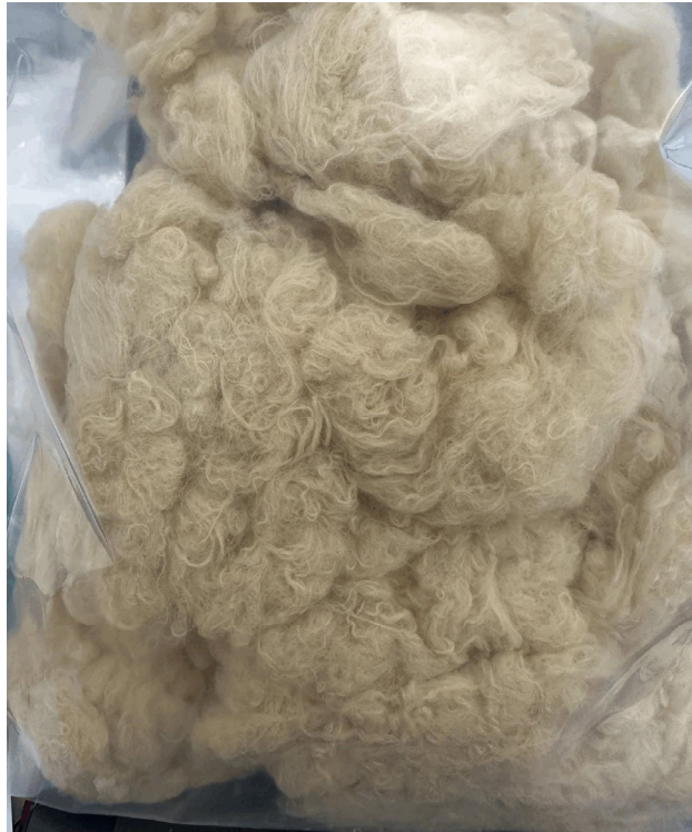
Figure [ ] : RENOA Staple Fiber After Cutting and Crimping
