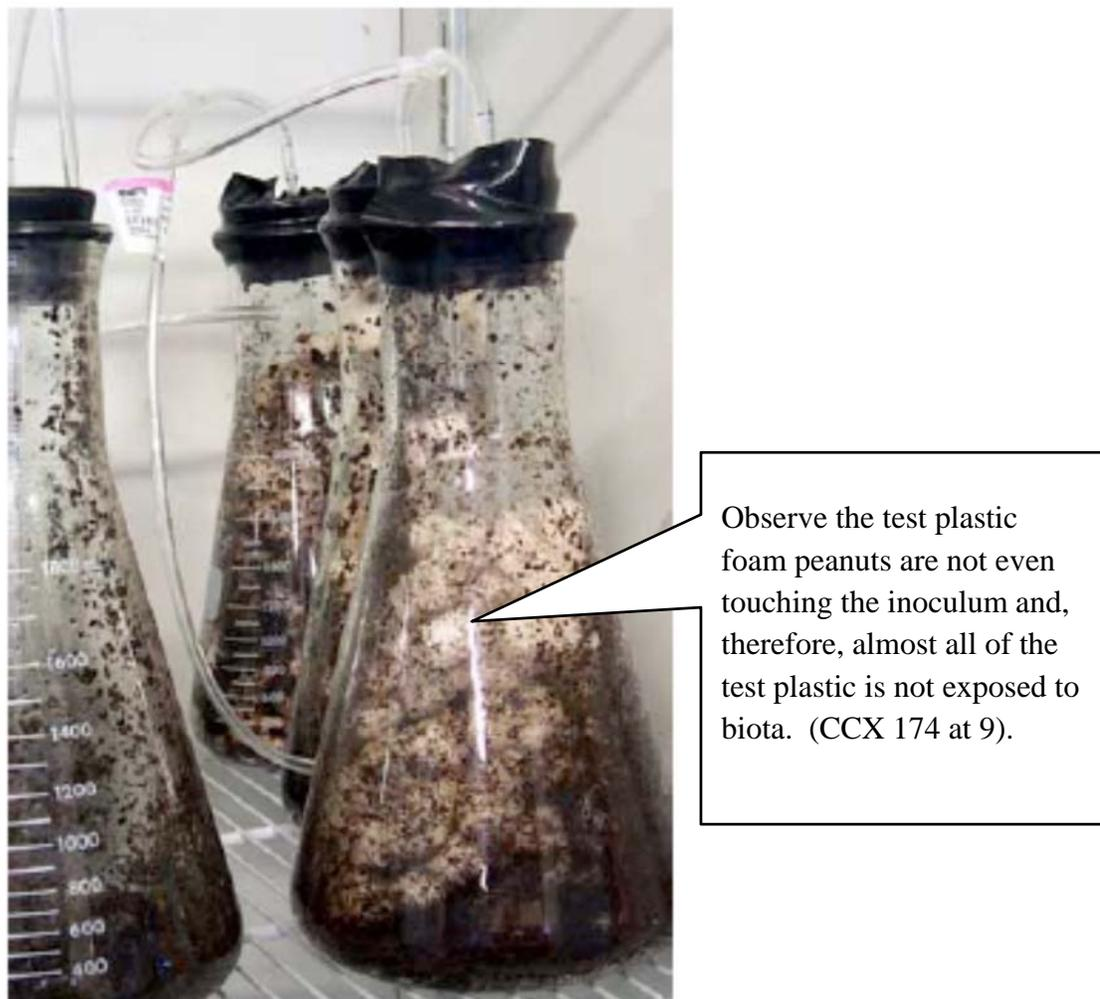
Figure 2. Thermophilic Composting Apparatus
