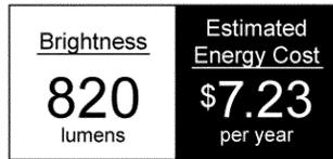
\* Minimum size for vertical label is 1.6" x 0.75". Scale label and all text proportionally.
