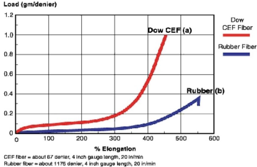
And last, since Dow CEF has a low but significant level of crystallinity at room temperature, CEF exhibits higher tensile set (lower elastic recovery) than rubber when extended to greater than 100% elongation. The 5-cycle tensile set measurement (Figure 11, page 15) shows this contrasting behavior between CEF and rubber fiber. The permanent set of CEF is a direct manifestation of its crystallinity and stands in marked contrast to the low tensile set of rubber fibers.
