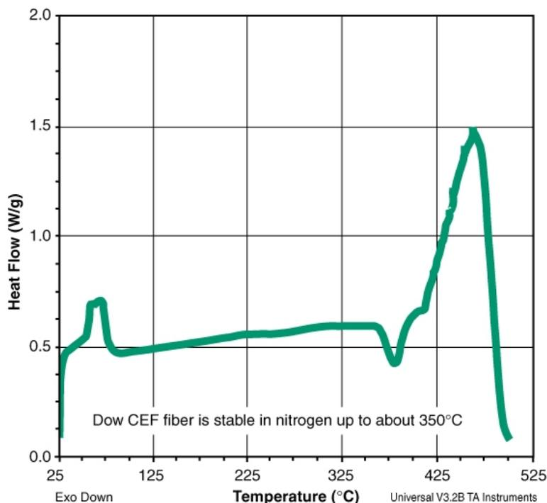
Furthermore, Figure 5, above, shows the heat stability of Dow CEF in nitrogen up to about 350°C.
