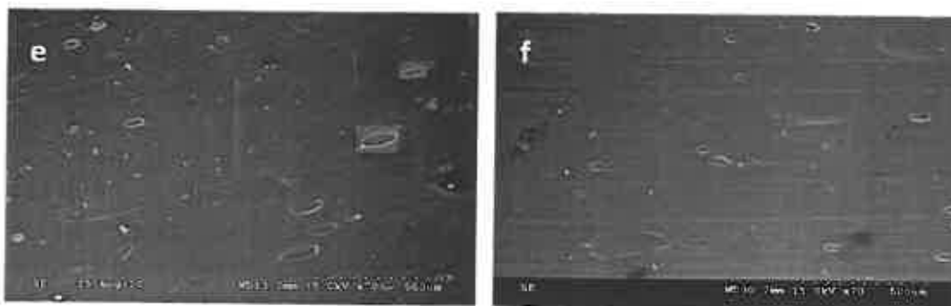
Figure 4. Scanning electron micrograph analysis of polypropylene amended with 2% ECM additive after 0 days (left) and 2 years (right) of soil incubation.
